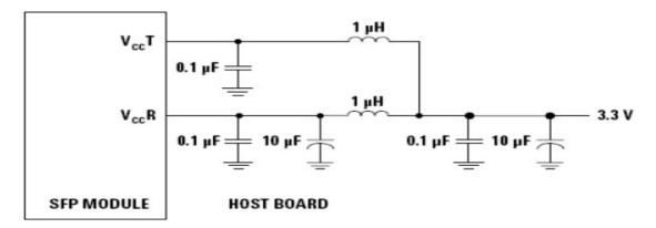
Note: Inductors with DC resistance of less than  $1\Omega$  should be used in order to maintain the required voltage at the SFP input pin with 3.3V supply voltage. When the recommended supply filtering network is used, hot plugging of the SFP transceiver module will result in an inrush current of no more than 30 mA greater than the steady state value
