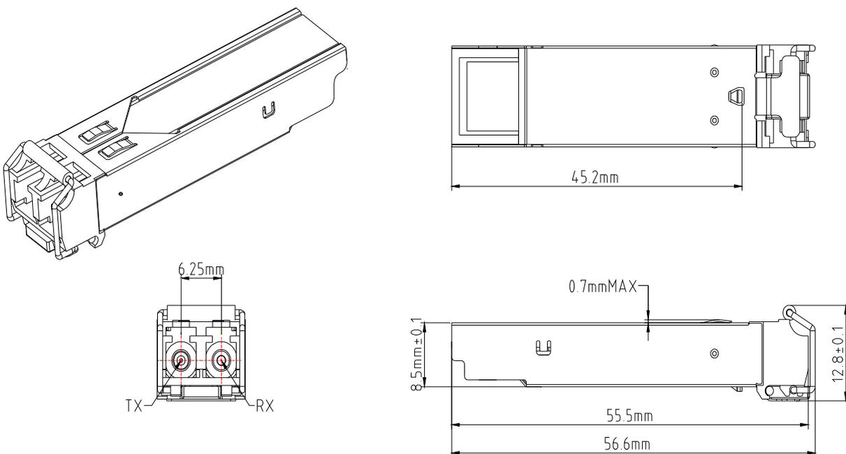
**[2.5Gb/s SFP Optical Transceiver with DDMI \(PTP8883D-3\)](#)**
